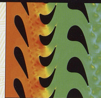
Simulation of a one-and-a-half stage turbine. Color corresponds to temperature. Such simulations pinpoint likely blade hot spots, which helps in the design of cooling conduits and blade coatings.
