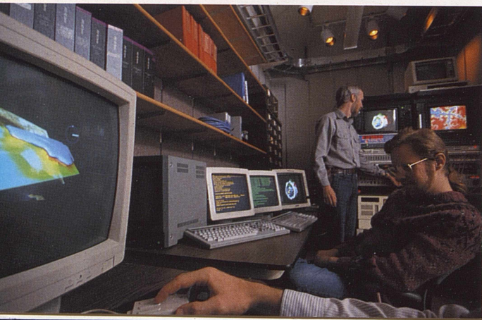
Joel Welling (standing) and Chris Nuuja of the Center's graphics group in the expanded new graphics lab. New hardware includes a Silicon Graphics Personal Iris, two Sun Sparcstations, an IBM System/6000 workstation and a rack of animation equipment.
